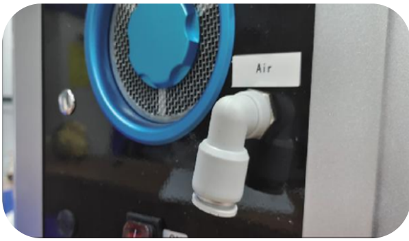
7. Insert the Air pipe into the all-in-one machine
