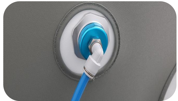
10. Insert the oxygen tube (blue) into the cabin
